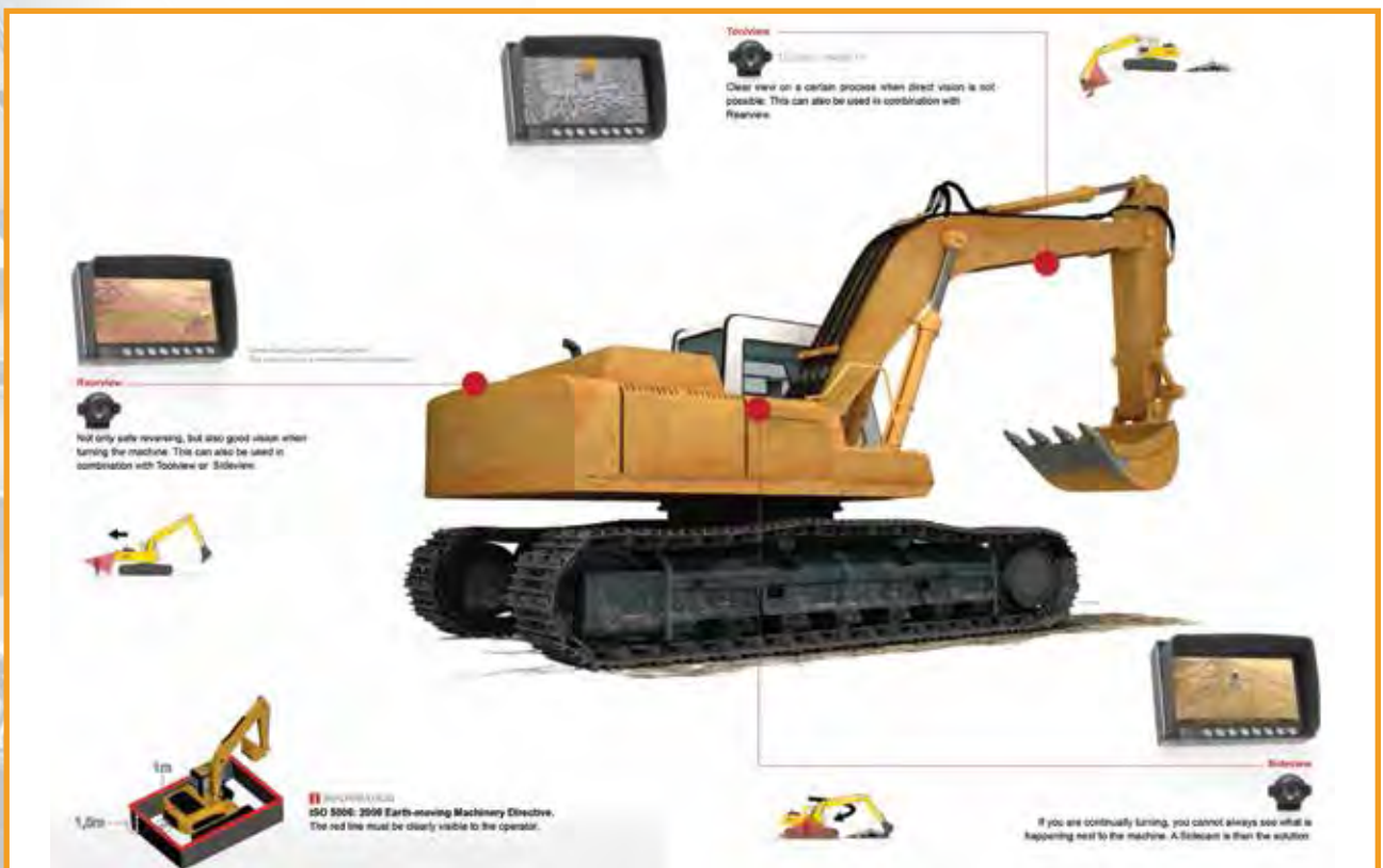
CCTV application on an excavator
