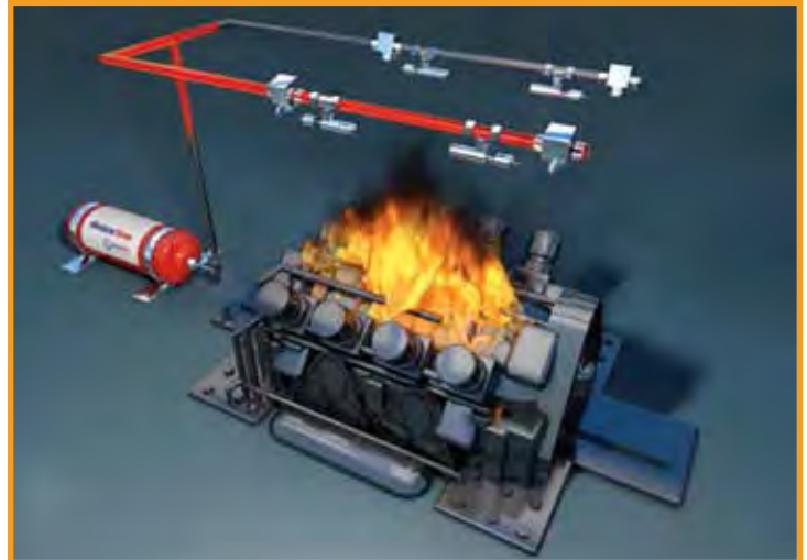
Detexline fire suppression system
